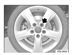
Turn wheel until adjustment screw is visible in threaded hole.
