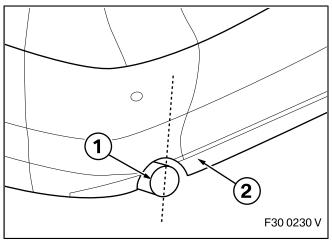
Push the Torca clamp **B** over the pipe (1) on the M Performance silencer **A**.
