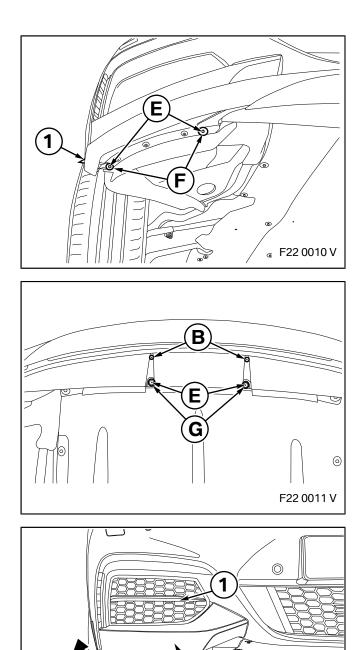
Remove the protective film (1). Screw in screws  ${\bf E}$  together with washers  ${\bf F}.$
