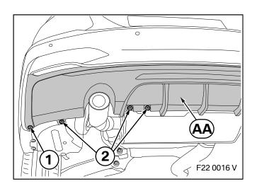
Place rear diffuser **AA** on the car and press it into place. Press in the plastic rivet (1) and tighten the screws (2).
