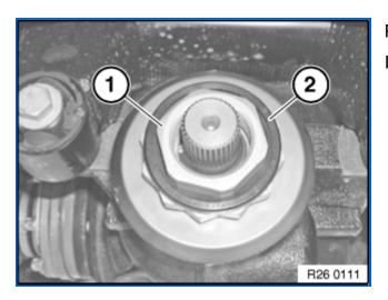
Place insert nut (1) with seal in insert collar of flange nut. Install retaining clip (2).
