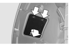
2. If necessary, pull the inside trim of the wheel house slightly inward. Turn the bulb holder counterclockwise and remove.
