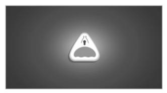
Pull the handle inside the cargo area. The trunk lid unlocks.
