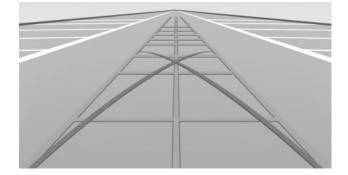
2. Turn the steering wheel to the point where the pathway line covers the corresponding turning circle line.
