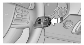
Press the button on the wiper lever.
