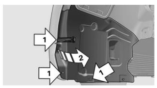
Pull off the bulb connector, arrow 1. Turn the bulb, arrow 2.
