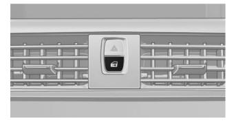
Pressing the buttons locks and unlocks the doors and the trunk lid when the front doors are closed, but they are not secured against theft.
