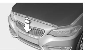
Let the hood drop from a height of approx. 16 in/40 cm and push down on it to lock it fully.
