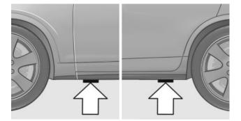
The jacking points for the vehicle jack are located at the positions shown.
