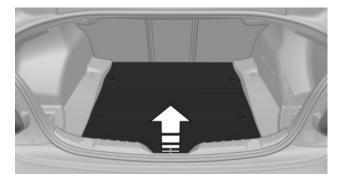
The screw-in tow fitting should always be carried in the vehicle. It can be screwed in at the front or rear of the BMW. It is stored in the onboard vehicle tool kit in the cargo area under the cargo floor panel.
