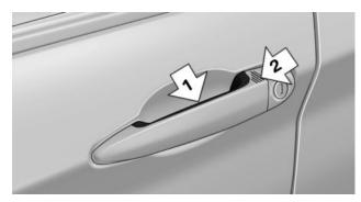
Grasp the door handle on the driver's or front passenger door completely, arrow 1.
