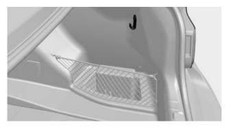
A multi-function hook is located on each side of the cargo area. The multi-function hooks can be loaded up to a max. of 8.8 lbs/4 kg.
