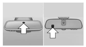
Photocells are used for control:
