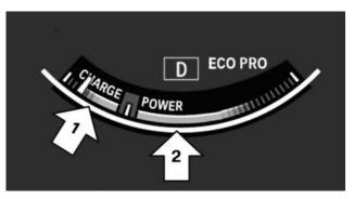
In the tachometer, a mark in the bar display indicates the current efficiency of the driving style. Mark in the CHARGE area, arrow 1: display for energy recovered by coasting or when braking.
