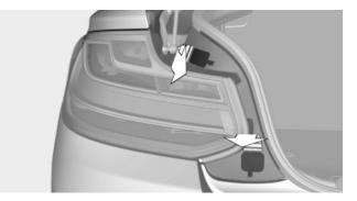
3. With the handle of the screwdriver from the onboard vehicle tool kit, loosen and remove the nuts on the two fasteners. Make sure that the nuts do not drop into the bumper area. In addition to the two outer fasteners, there is another inner fastener.
