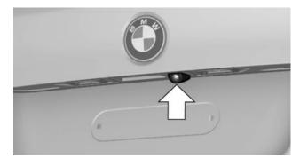
The camera lens is located in the handle of the trunk lid. The image quality may be impaired by dirt.
