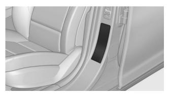
These pressure values can also be found on the tire inflation pressure label on the driver's door pillar. Maximum permissible speed
