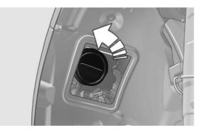
2. Tilt the bulb down and then up to loosen it from the holder and remove.
