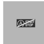
The display indicates that the conditions for an automatic engine stop have not been satisfied.
