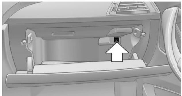
The USB interface is located in the glove compartment.
