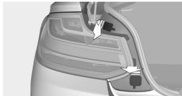
3. With the handle of the screwdriver from the onboard vehicle tool kit, loosen and remove the nuts on the two fasteners. Make sure that the nuts do not drop into the
