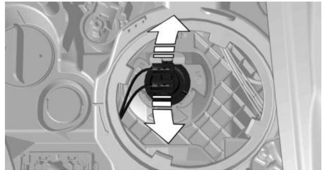
3. Pull the connector off the bulb.
