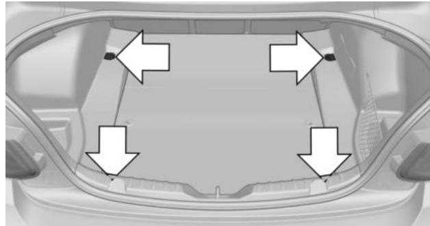
To secure the cargo there are two or four lashing eyes in the cargo area.
