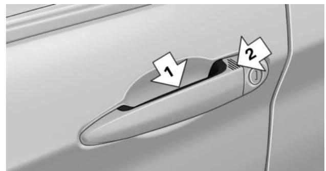
Grasp the door handle on the driver's or front passenger door completely, arrow 1.
