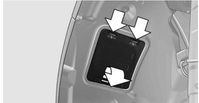
2. If necessary, pull the inside trim of the wheel house slightly inward. Turn the bulb holder counterclockwise and remove.
