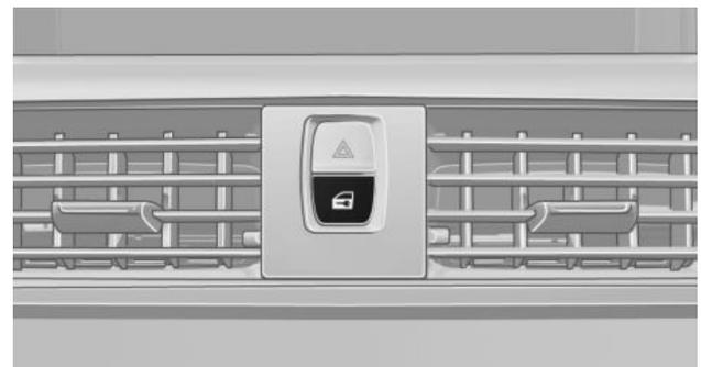
Via the button for the central locking system. If the vehicle has been locked from inside, the fuel filler flap remains unlocked.
