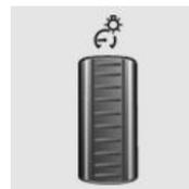
The parking lamps or low beams must be switched on to adjust the brightness.
