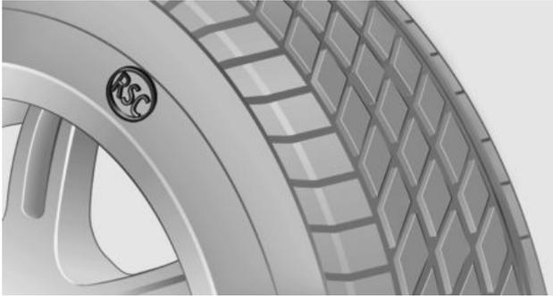
RSC label on the tire sidewall.
