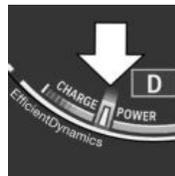
The mark in the bar display below the tachometer is backlit in blue and is located at the zero point. The tachometer approximately indicates idle speed.
