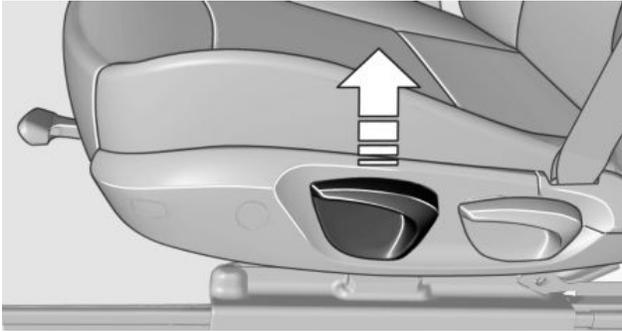
Pull the lever and apply your weight to the seat or lift it off, as necessary.
