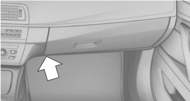
The socket is located below the glove compartment.
