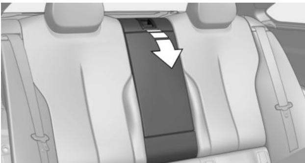
Reach into the recess and pull the middle section forward.
