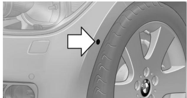
The ultrasound sensors for measuring parking spaces are located on the wheel arches.
