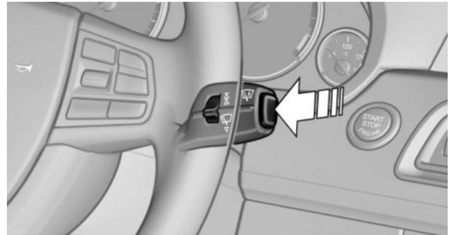
Press the button on the wiper lever.
