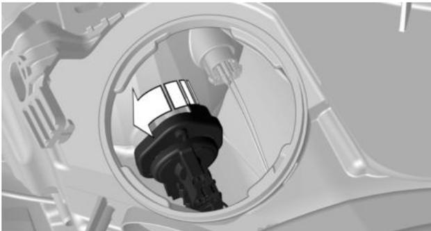
2. Install the new bulb in reverse order of removal. Turn the clockwise bulb here until it hits the stop.
