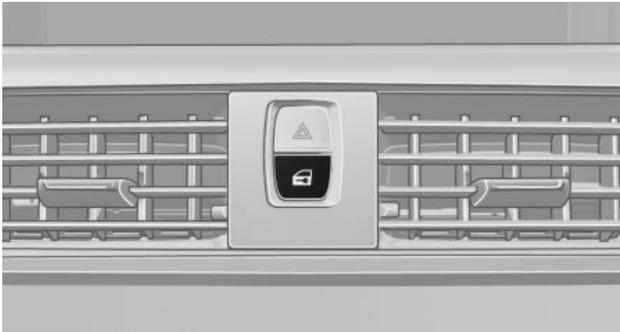
Pressing the buttons locks and unlocks the doors and the trunk lid when the front doors are closed, but they are not secured against theft.
