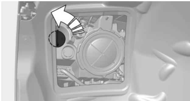
2. Press the bulb gently into the socket, turn counterclockwise and remove.
