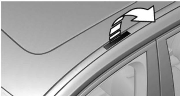
The anchorage points are located in the roof drip rail above the doors.
