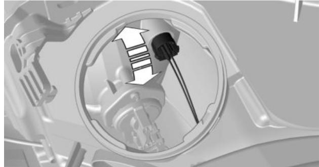
2. Carefully remove the bulb from the bulb holder.
