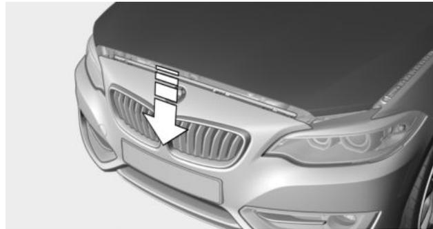
Let the hood drop from a height of approx. 16 in/40 cm and push down on it to lock it fully.
