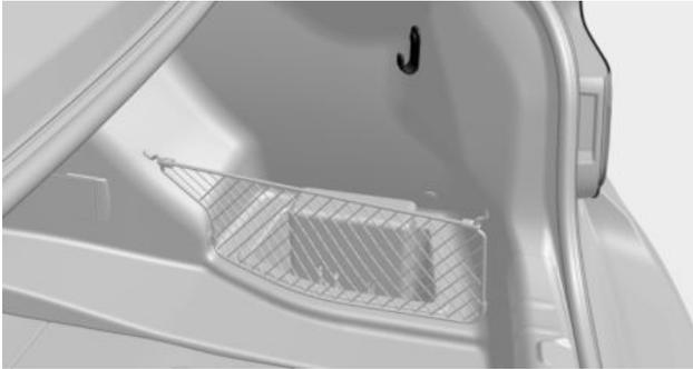
A multi-function hook is located on each side of the cargo area. The multi-function hooks can be loaded up to a max. of 8.8 lbs/4 kg.
