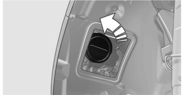
2. Tilt the bulb down and then up to loosen it from the holder and remove.
