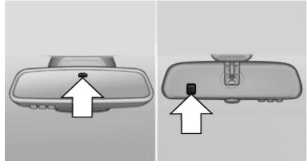
Photocells are used for control:
