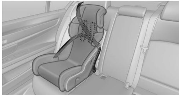
The rear safety belts and the front passenger safety belt can be locked against pulling out for mounting the child restraint fixing systems.
