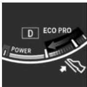
The arrow indicates that the driving style can be adjusted to be more fuel efficient by backing off the accelerator for instance.
