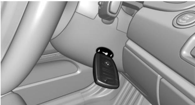
Automatic transmission: if a corresponding Check Control message appears, hold the remote control, as shown, against the marked area on the steering column and press the
