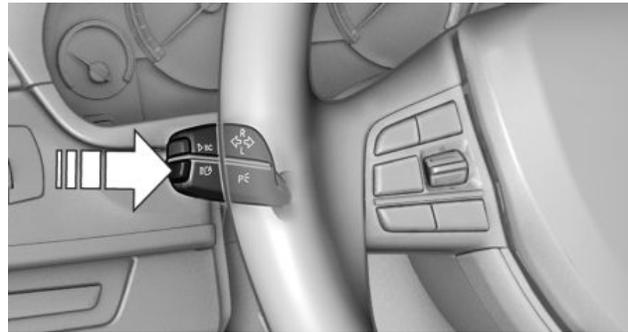
The High-beam Assistant can be activated when the low beams are switched on.
