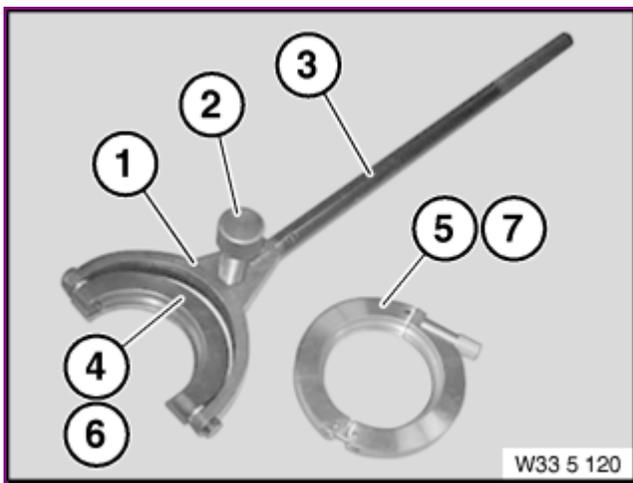
Note: For removing and installing output shaft in rear axle final drive.
