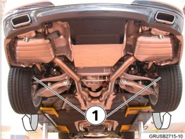
Hold the front driveshaft and manually spin the rear wheels (1). The rear driveshaft needs to spin.
