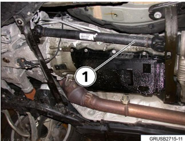
If the front driveshaft (1) cannot be held steady with minimal effort – the internal clutch pack is seized (extreme overheat).
